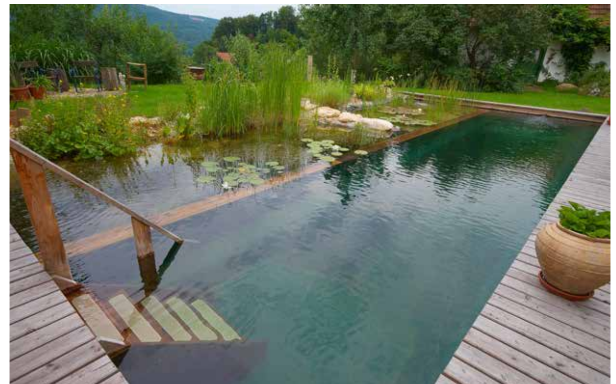
Natural beauty A normal pool can be transformed into a self-cleaning one by incorporating a planted area – the so-called regeneration zone – either within the existing structure of the pool or by extending the water surface. Natural Pools UK ( naturalpoolsuk.com ) uses technology by Austrian brand Biotop ( biotop-natural-pool.com ) to carry out conversion projects of this kind, as well as to create dream pools from scratch. ►
